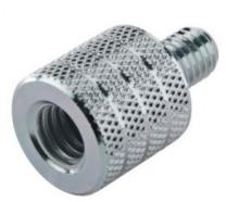
Thread adapter with an external diameter of 18 mm x 30 mm. Female thread of 3/8". Male thread M8 x 12 mm.
