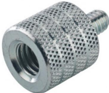
Thread adapter with an external diameter of 18 mm. Female thread 3/8". Male thread 1/4".
