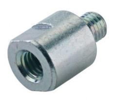
Thread adapter with an external diameter of 20 mm. Female thread 3/8". Male thread M 10 mm. With a width across flats of 17.
