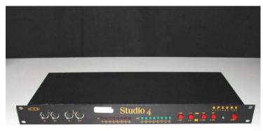
The Opcode Studio 4 is a 128 channel, 8-IN/8-OUT MIDI interface/SMPTE synchronizer. As an interface, the Studio 4 allows the Macintosh to independently communicate with each of the 8 MIDI INs and OUTs. As a synchronizer, it reads and writes SMPTE in all formats. Opcode's Open Music System (OMS) software adds filtering, channelization, note range splitting, controller mapping, and velocity and control value modification to the Studio 4's capabilities.
