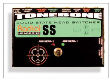
The Radial Headbone is a specially designed switching device that lets you toggle between two different guitar amplifier heads using a single speaker cabinet. With the Headbone in your rig, you can use your Marshall head for rhythm and your Mesa-Boogie head for soloing. This is of particular interest for players that demand the utmost in tonal performance when on stage or in the studio.
