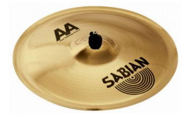
SABIAN AA cymbals are made from 80% copper and 20% tin. During manufacturing, the blanks are rolled in up to 8 different directions, which lends the cymbal its great flexibility. The cymbal's bell and curvature are pressed into the flat, disc-shaped blank in a press. The cymbal is subsequently machine hammered and lathed by hand. This is how each cymbal gets its individual sound characteristics.
