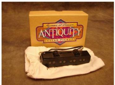
The neck position is wound "top going" and North polarity. When used in combination with the bridge pickup will be hum-canceling. Both pickups have the traditional pole spacing. The magnets are protruding from the top and bottom of the flatwork for a smooth even response. Each pickup is recreated to fit in your old classic and comes with black aged pickup cover, schematic, and mounting screws. Hookup wire is the classic "push back" c braid wire.
