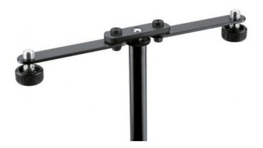
The flexible microphone bar for microphone stands. Two moveable bars position the microphone where ever you would like it. Each bar is fitted with a captive knurled screw. The entire bar can be screwed onto all standard microphone stands with a 3/8" threaded connector.
