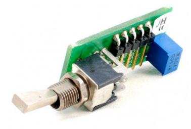
The PA2 is a straight booster preamplifier mounted on a minitoggle switch. Perfect if you want to just plain overdrive the input of your amp for distortion. It has a trim pot so you can preset the amount of boost up to an additional 20 dB. The PA2 will also work with passive pickups.
