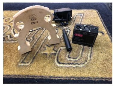
AKG "DB1" PONTICELLO AMPLIFICATO PER CONTRABBASSO CON PHANTOM POWER E ALIMENTATORE
