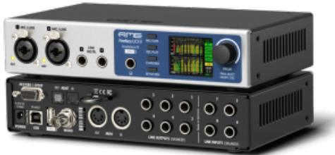
Interfaccia Audio USB fino a 192 kHz, 20 In/Out: 8 x Analog I/O, 2 x Preamp Mic/inst controllati digitalmente, 2 x Line / Inst. In, ADAT I/O, SPDIF e AES/EBU I/O, Word Clock e MIDI I/O
