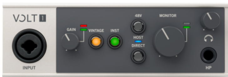
Interfaccia audio 1-in/2-out USB 2.0
