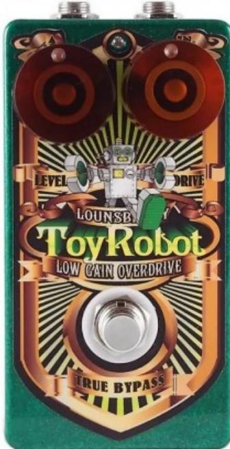
Handwired Point-to-Point "Toy Robot" multi stage analog FET low gain overdrive
